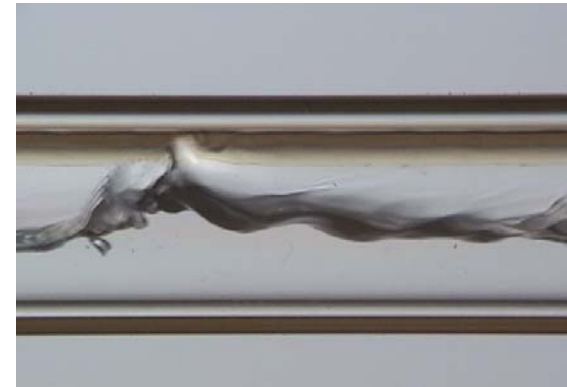
i) 250 kg/m 2 s mass flux, 10% quality
