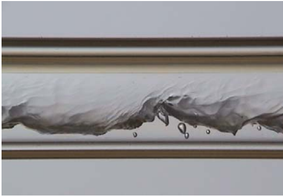
d) 125 kg/m 2 s mass flux, 50% quality
