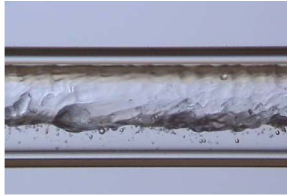
k) 250 kg/m 2 s mass flux, 20% quality
