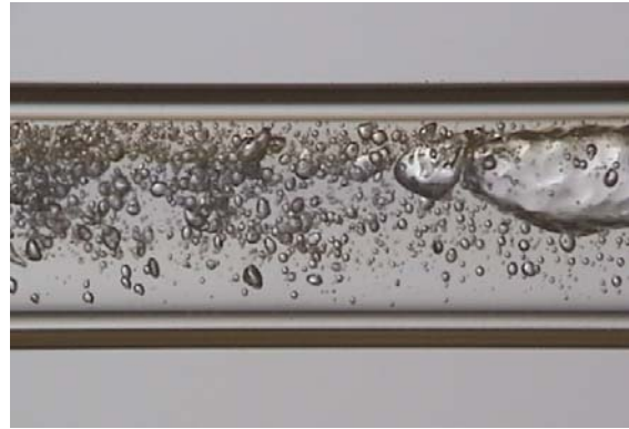
e) 125 kg/m 2 s mass flux, 50% quality
