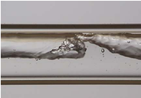
h) 250 kg/m 2 s mass flux, 10% quality
