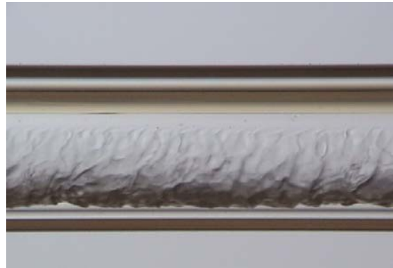
g) 125 kg/m 2 s mass flux, 95% quality
