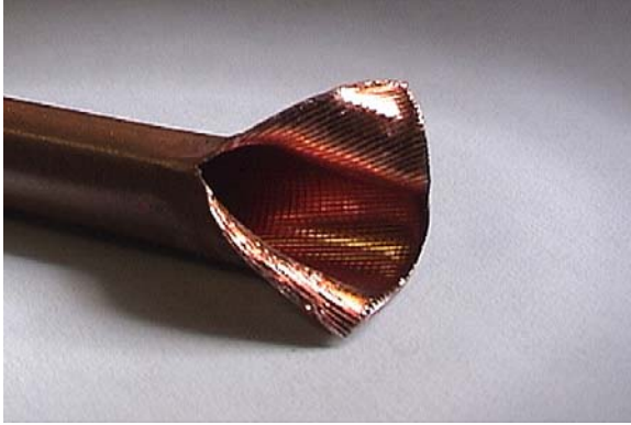
Figure 1.3. Internal geometry of helically microfinned tubing
