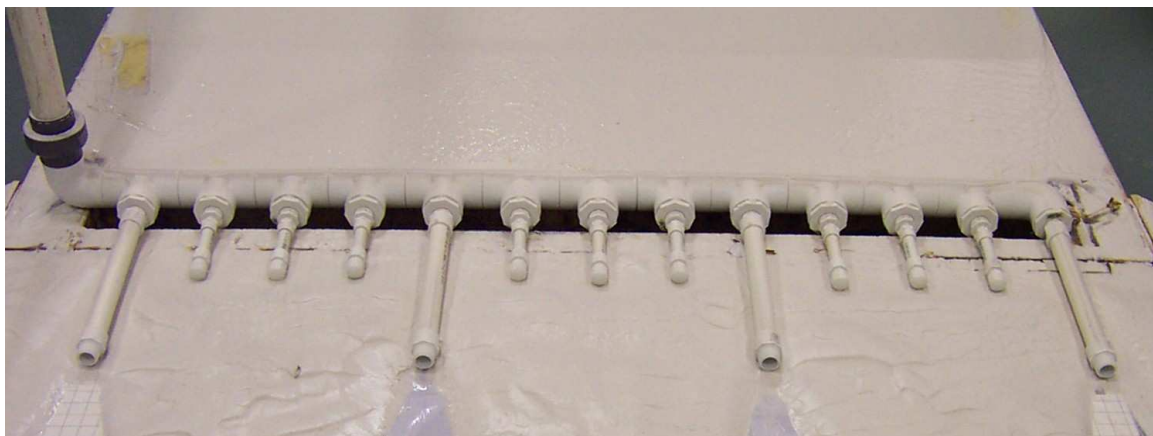
Figure 3-29 Manifold for circular wall jet experiments showing a configuration of 4 jets. The manifold allows up to 13 jets changing jet diameter, jet separation, and diffuser lengths. The jets having shorter diffuser lengths are not taking part of the test showed in the picture, they are closed.
