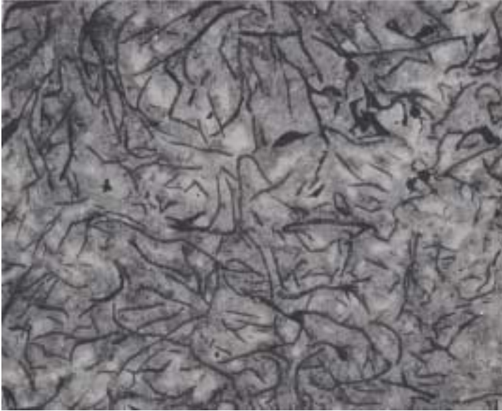
Figure 25. Typical microstructure of gray iron (100 ×), dark graphite flakes in a surrounding matrix of 20 % free ferrite (light constituent) and 80 % pearlite (dark constituent) (Shackelford, 1988)
