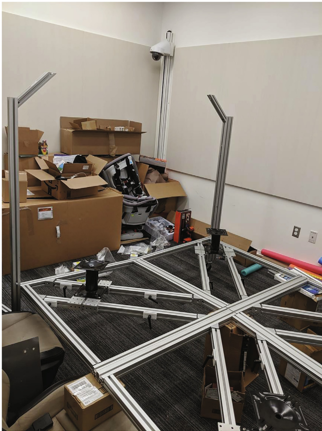
Fig. 3. Rail system with pedestals that allow seats to be rotated as well as translated.
