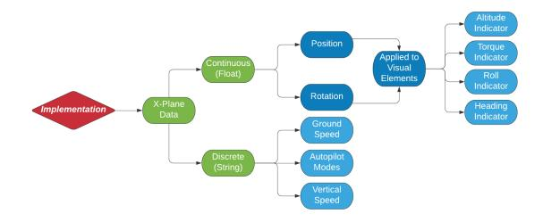
An example of discrete behavior is the autopilot mode display of the HUD. Depending on the signal from X-Plane, a different string will occupy the field for the collective, roll, or pitch fields as can be seen in Figure 18. These values are discrete and typically limited, so that the number of possible values displayed is fixed.
