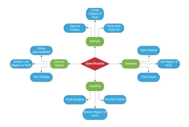
In the example specification shown in Figure 10, four elements are identified: attitude, airspeed, heading and groundspeed.
