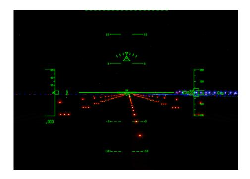
HUD images are projected at a focal distance such that visual accommodation time, or the time needed to switch focus from flight instruments to the outside environment, between HUD information and the outside environment is minimized [31].
