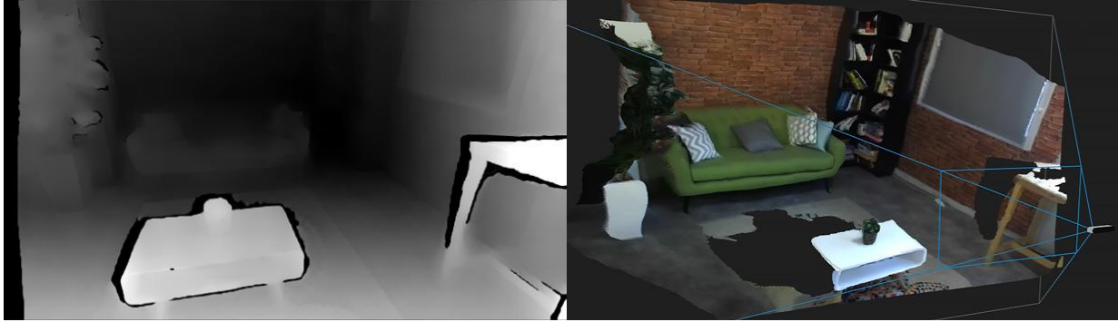
Figure 16. The depth and point-cloud maps
