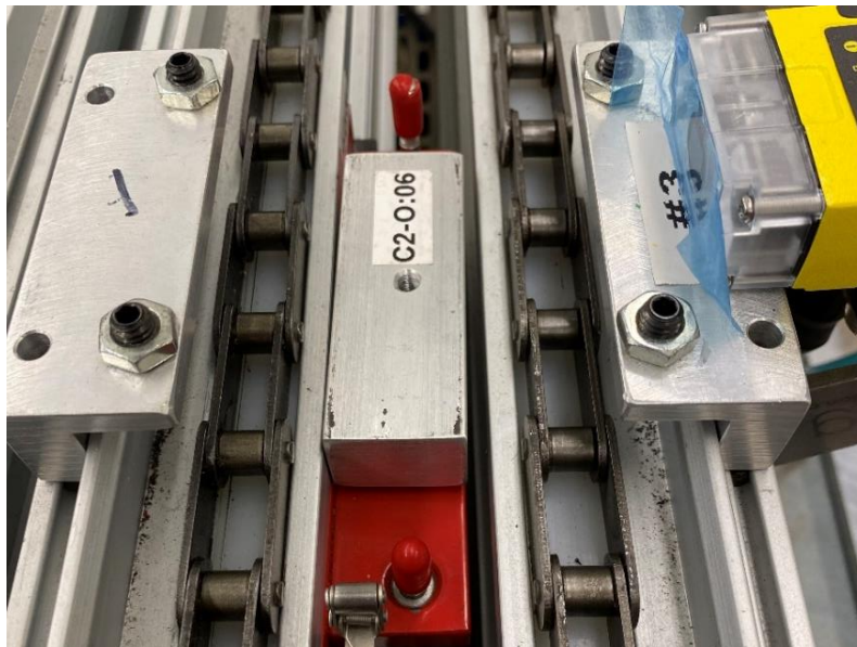
Figure 36. Linear actuator for the main conveyor
