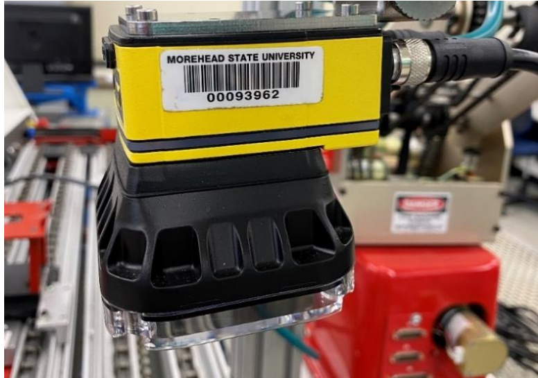
Figure 38. Cognex® machine vision camera sensor
