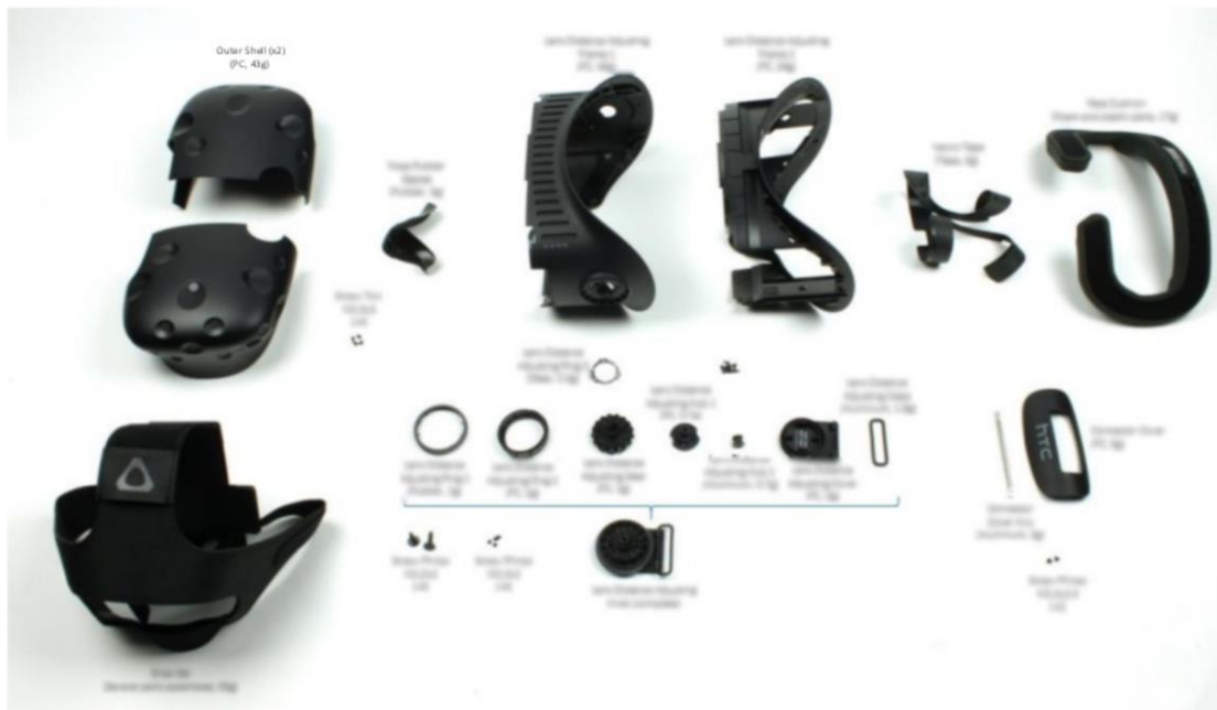
Figure 6. Part collection for a Vive® VR HMD
