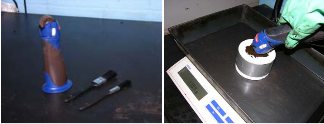
Figure 3-3. Tools for applying tack coat.
