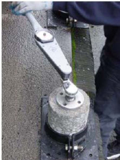
Figure 2-9. Torque bond test (Tashman et al. 2006).
