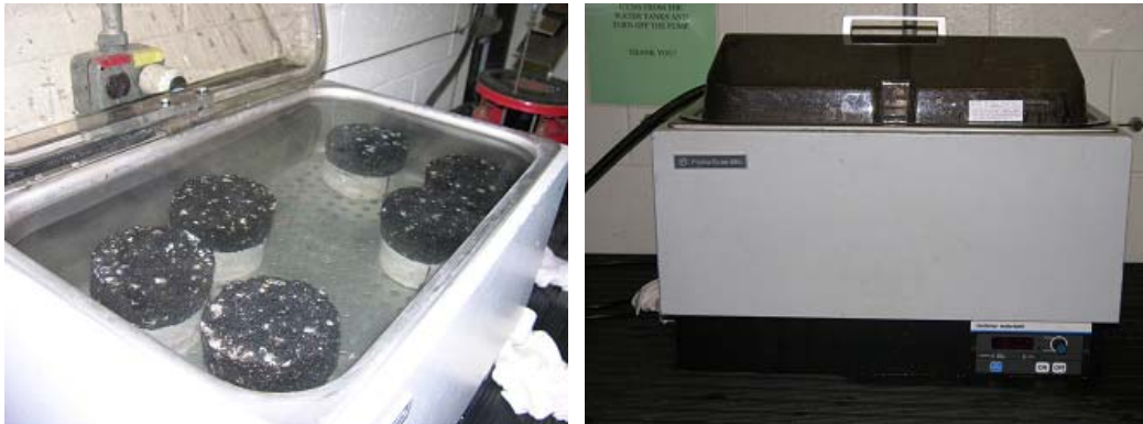
Figure 3-5. Partially vacuumed HMA-PCC specimens in a 140 °F (60 °C) water bath.
