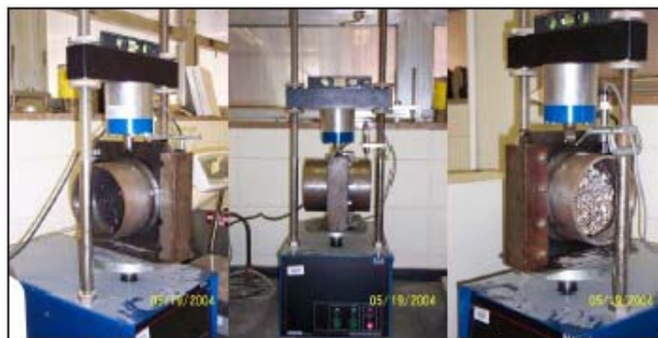
Figure 2-7. Laboratory bond interface strength device, LBISD (Woods, 2004).
