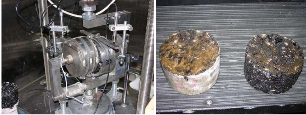
Figure 3-6. Moisture conditioned HMA-PCC specimen during testing and after failure.
