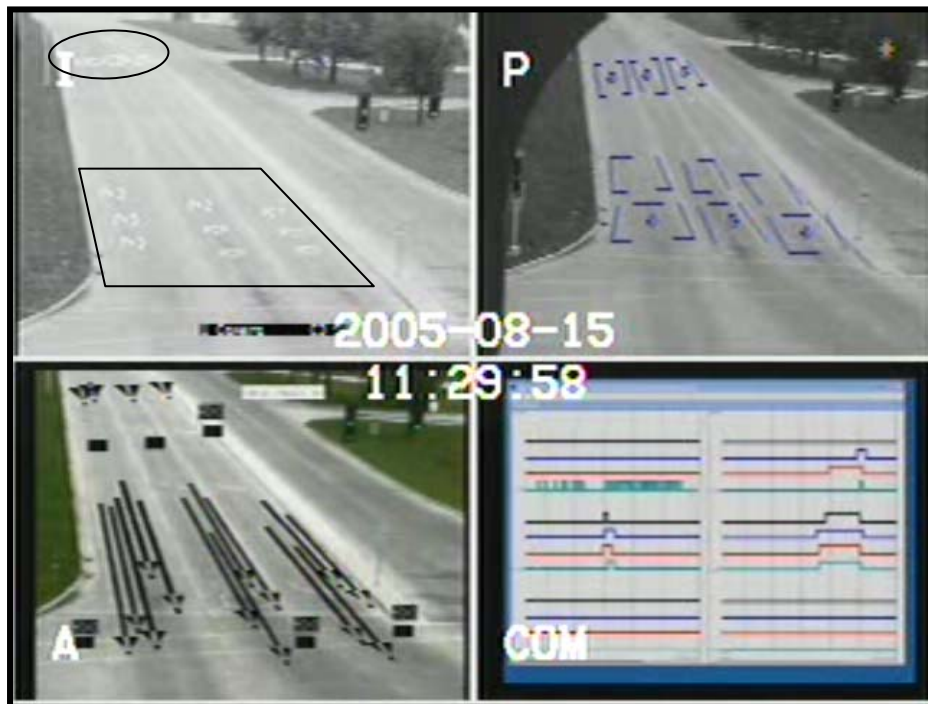
Figure 4-5. Configuration of VD zones in initial setup.
