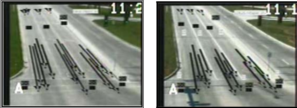
Figure 5-2. Configuration setup 1 and setup 2 of Autoscope.
