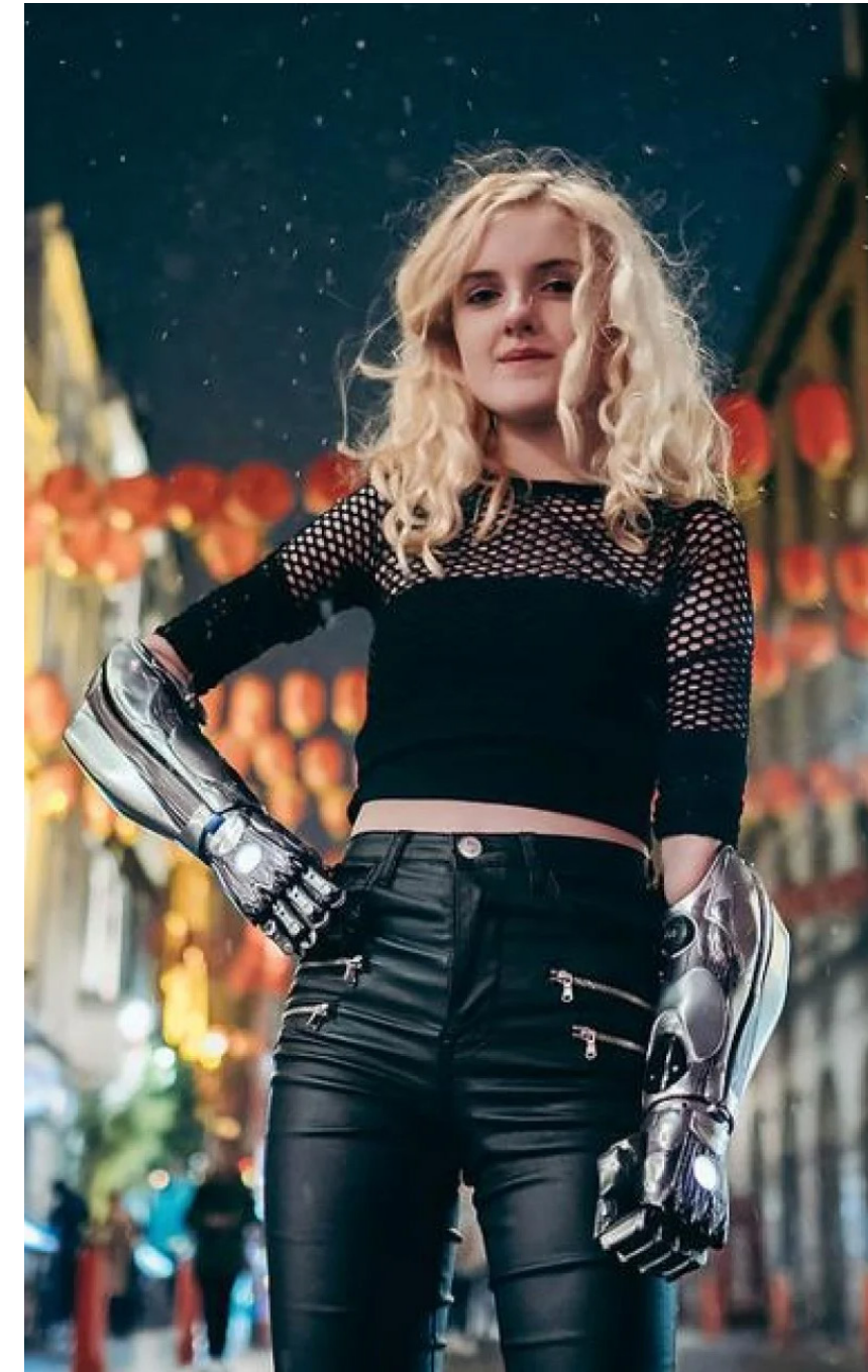
This is a photo of Open Bionics most advanced prosthetic, the Hero Arm, which relies upon myoelectric sensors to perform simple gripping functions. Despite its relative simplicity, it retains a similar size and shape regardless of the user’s age or body type.
