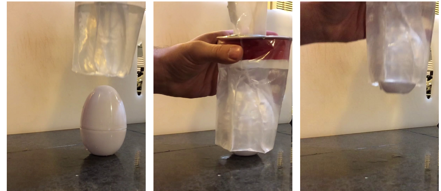
A flash prototype soft gripper made from plastic sheeting, cups, and water. It utilizes the change in volume of the water around an object in order to grip it while only applying a minimal amount of pressure to the object.
