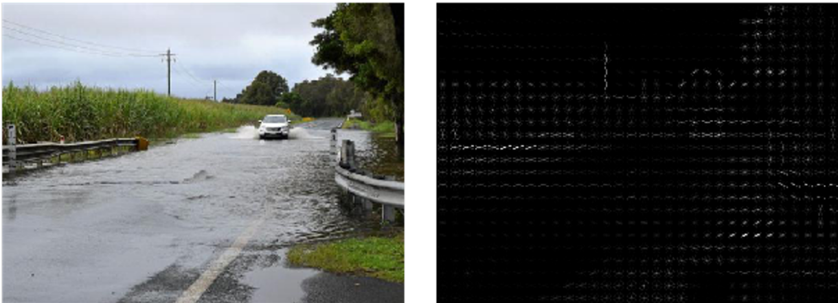
Figure 8. Sample image and its HOG feature descriptor
