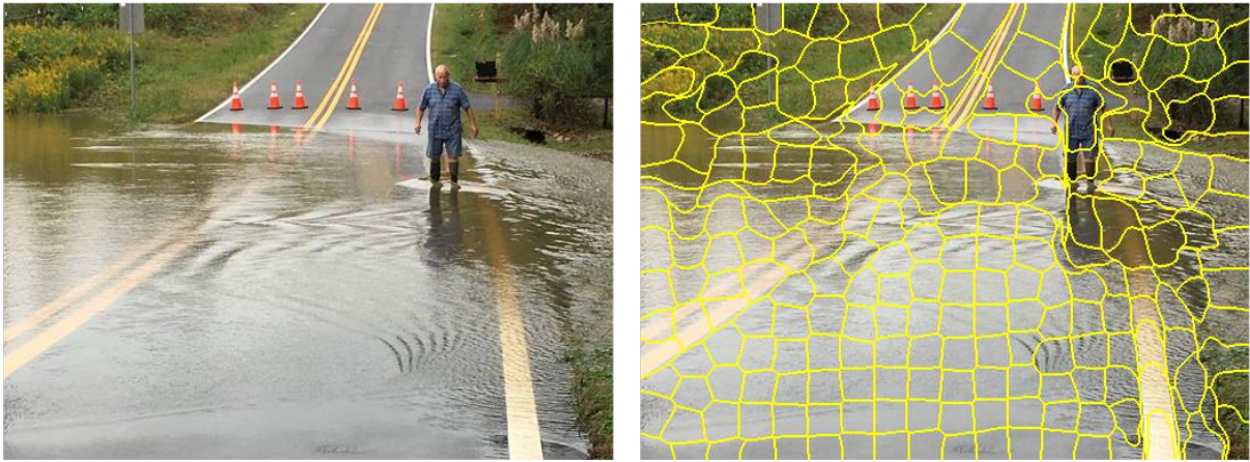
Figure 14. SLIC example: (left) Original image (right) Superpixels
