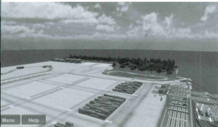
Figure 2. Shown here is a screen capture of computer simulation that models a sample port layout. The image is quite detailed in showing the travel lanes and loading area, container parking areas, gantry cranes, and the container ship.
