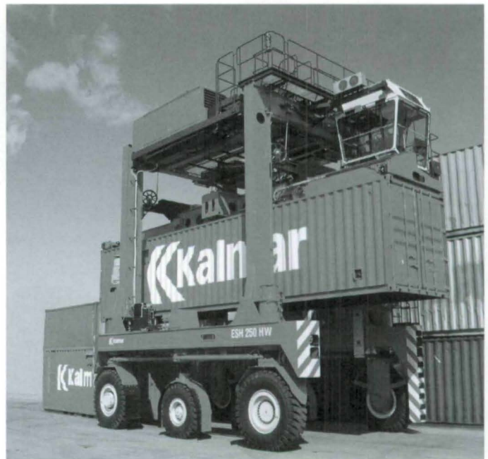
Figure 3. Kalmar ESC 350 shuttle or straddle carrier is used to move loaded or empty shipping containers from one location to another on the dock area. Simulation activities require that the operator perform tasks the same as would be necessary on the job. Tasks such as steering, throttle control, latching, and unlatching of containers must be performed. (Photo courtesy of Cargotec.)
