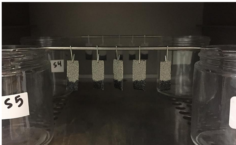
Figure 2.4. Picture of working electrodes in a vacuum oven.
