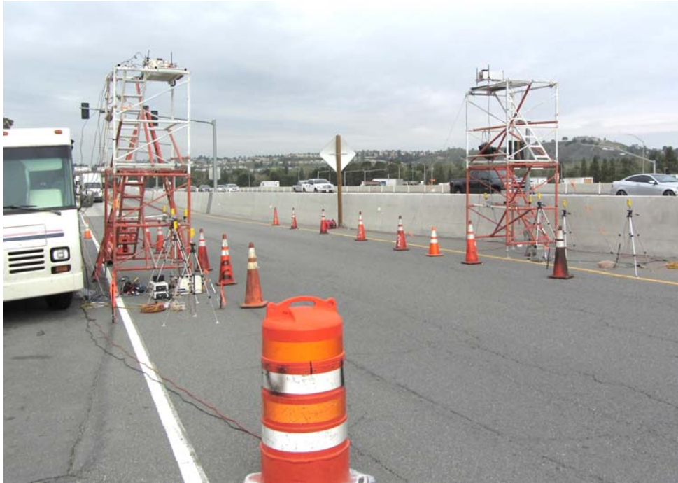
Figure S1. Photograph at the Peralta Weigh Station of the setup used to detect exhaust emissions from heavy and medium-duty trucks in 2017.
