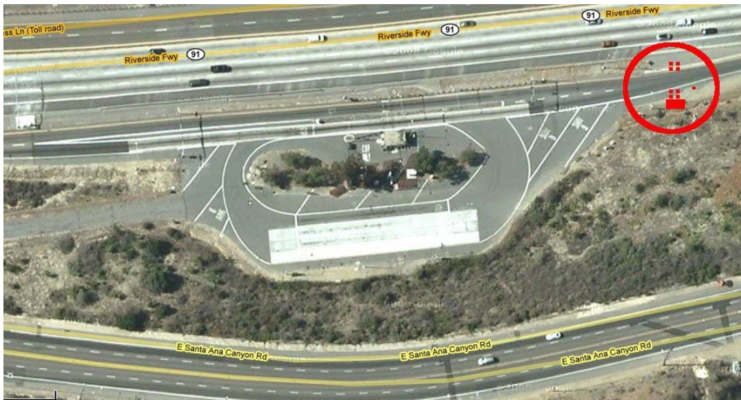
Figure S2. A satellite photo of the Peralta weigh station located on the Riverside Freeway (State Route 91). The scales are located on the inside lane next to the building in the top center and the outside lane is for unloaded trucks. The measurement location is circled at the upper right with approximate locations of the scaffolding, support vehicle and camera.
