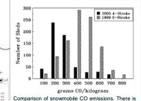
Comparison of snowmobile CO emissions. There is a shift in the distribution of about 40% lower for 4stroke sleds. Most of the tailing to higher values is from one brand of sleds.
