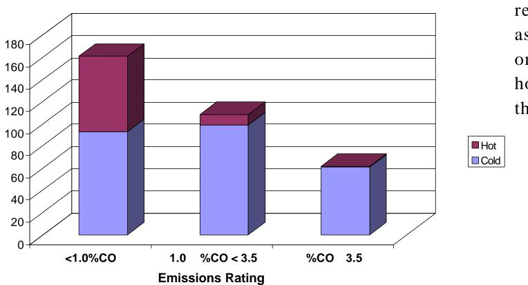
This graph shows the number of vehicles that received a GOOD, FAIR, or POOR rating, as well as if the vehicle was a cold or hot vehicle. Only one vehicle received both a POOR rating and was a hot vehicle from both days of measuring vehicles at the high school.
