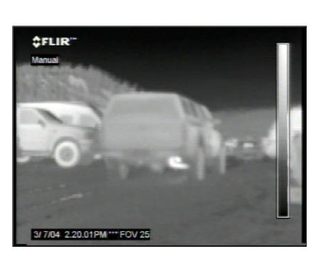
•Both of the vehicles in the IR images above are hot, however because snow does not reflect IR radiation, there is no reflection on the road from the underbody of the vehicles.
