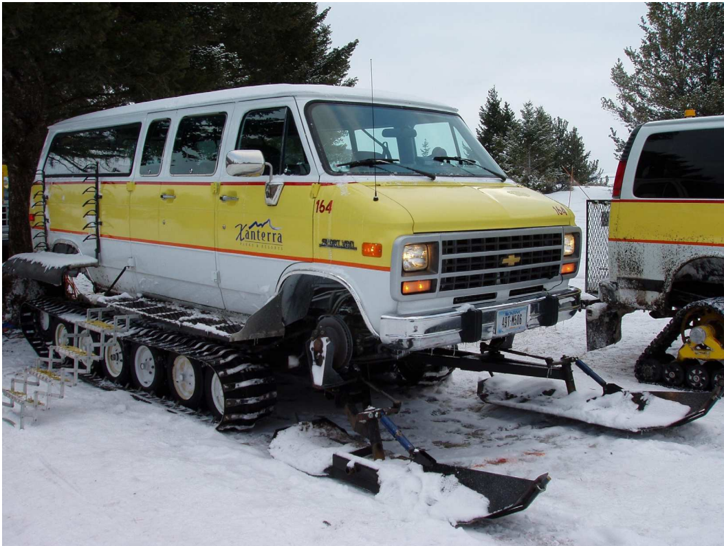
Figure 12. Xanterra 164 is a 1992 Chevrolet Van with a rear driven Snowbuster track/ski conversion.
