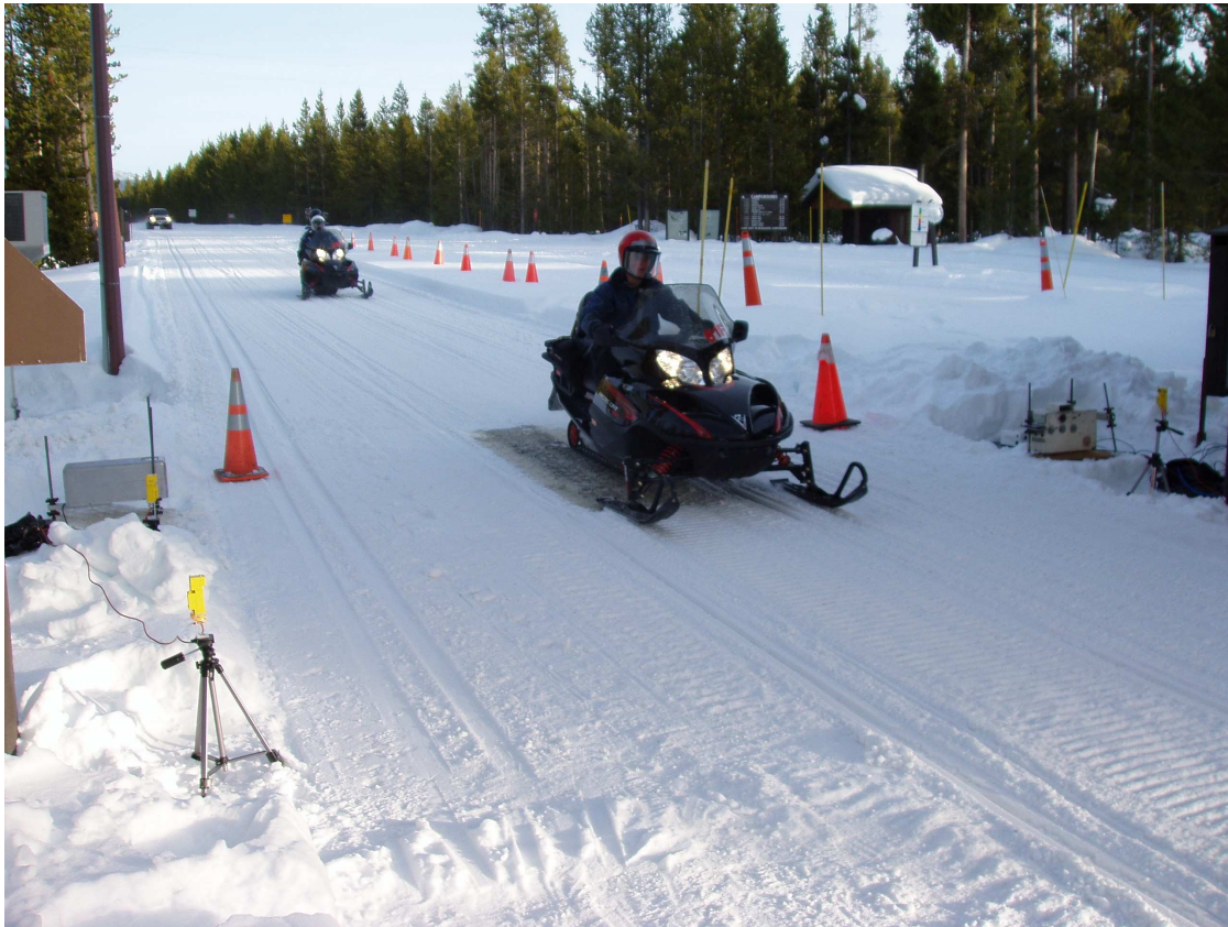
Figure 2. Photograph of a 2005 Arctic Cat snowmobile exiting Yellowstone National Park. The FEAT detector is in the upper right of the photo and opposite it is the IR/UV source. Underneath the first snowmobile is a plastic mat laid down in an attempt to eliminate excess snow spray.
