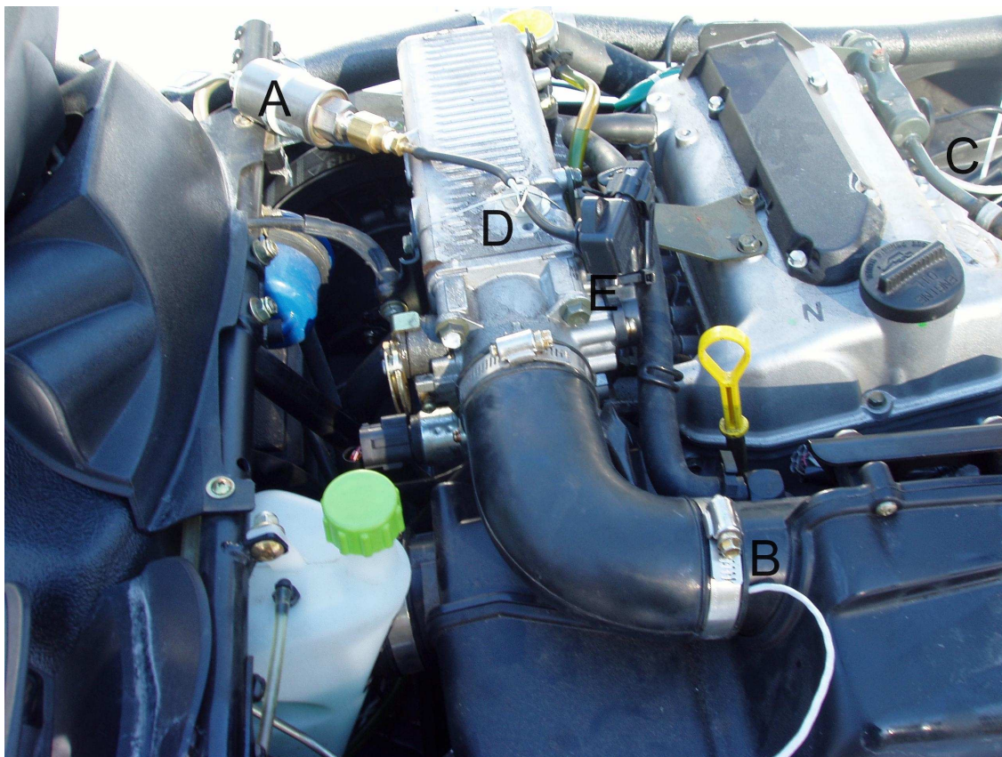
Figure 3. Arctic Cat engine showing the pressure transducer (A), thermistor (B), the top of the rpm optical pickup (C), the precision engineered rubber stopper and tee (D) for connecting the manifold pressure sensor (E) to the pressure transducer.
