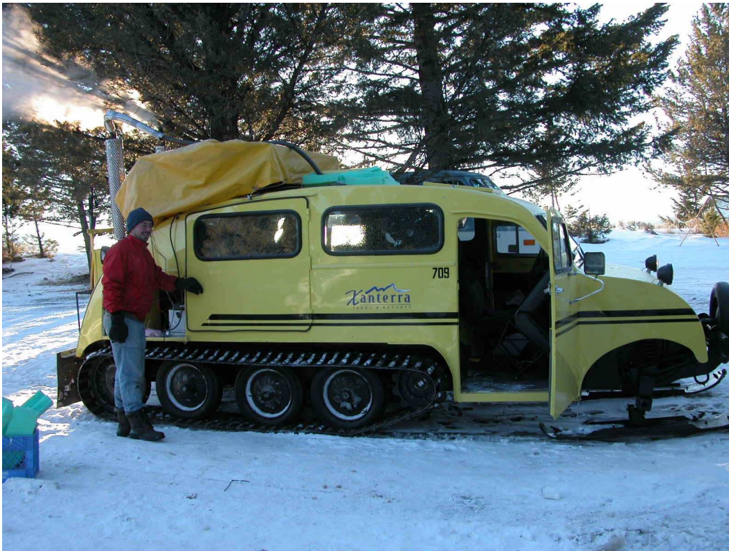
Figure 11. Vintage Bombardier 709 that utilizes a rear engine, forwards driven twin track and twin steering ski arrangement. This engine has an elevated exhaust system and the sample and data lines enter the cabin through a rear roof hatch.
