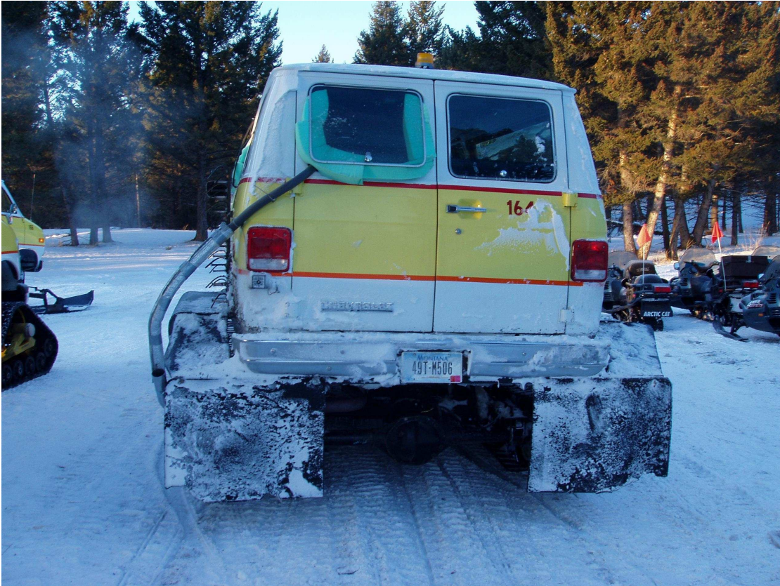
Figure 13. Rear view of a Snowbuster coach showing the tailpipe extension, insulated sample line and the temporary foam insulation installed to seal the rear window.
