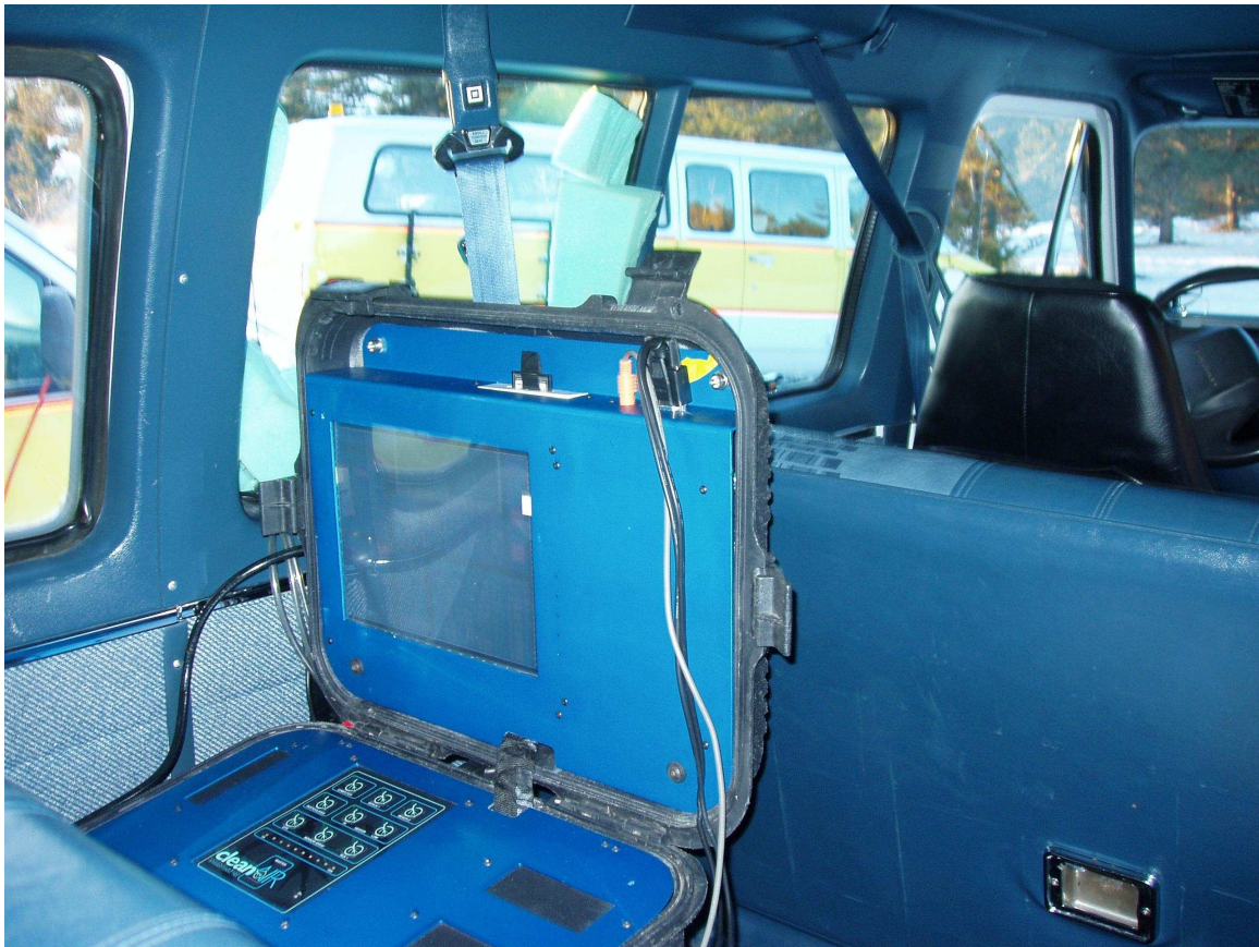
Figure 9. Photograph of the Montana system ready for sampling in a coach. Pictured are the video screen at left, compact flash card top center, GPS receiver connector top right and the exhaust lines exiting the cabin through the side window.
