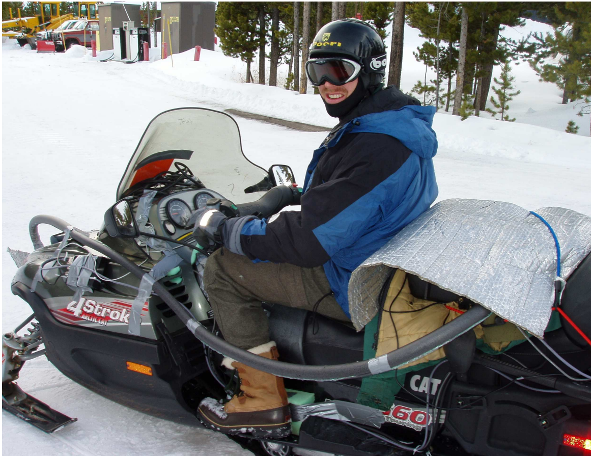
Figure 4. Arctic Cat snowmobile with the portable emissions in the rear passenger seat.
