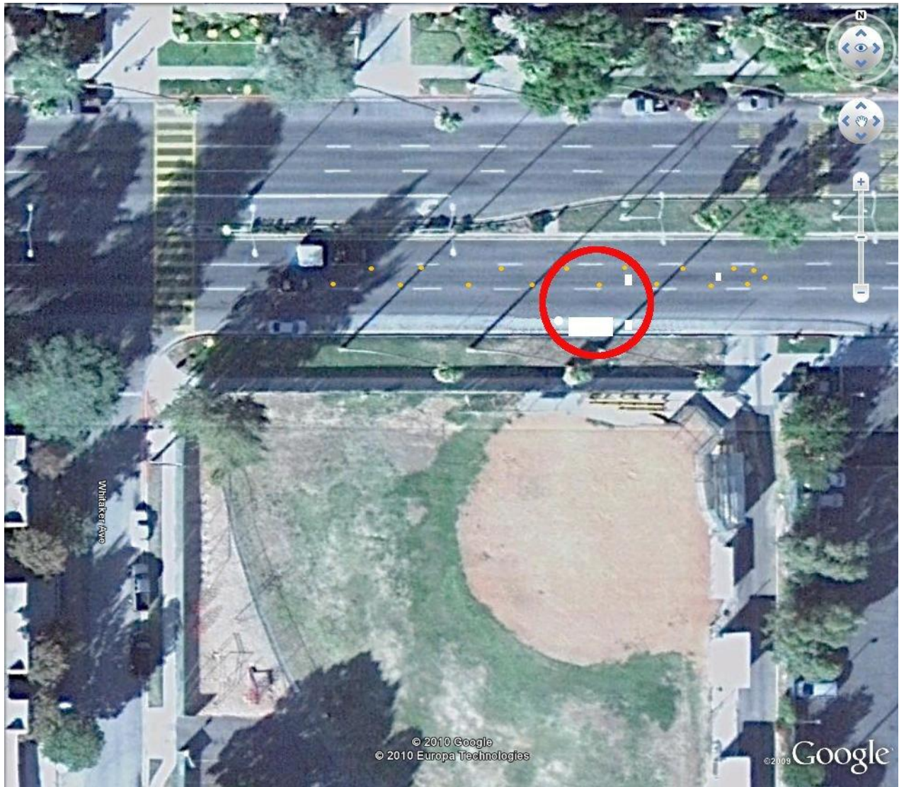
Figure 1. A satellite view of the Sherman Way monitoring location with Whitaker Ave. on the left edge of the picture. The location of the motor home, source, detector and camera are located inside the red circle. The source generator is located to the right of the source in the closed middle lane. The traffic cones are shown as yellow dots.
