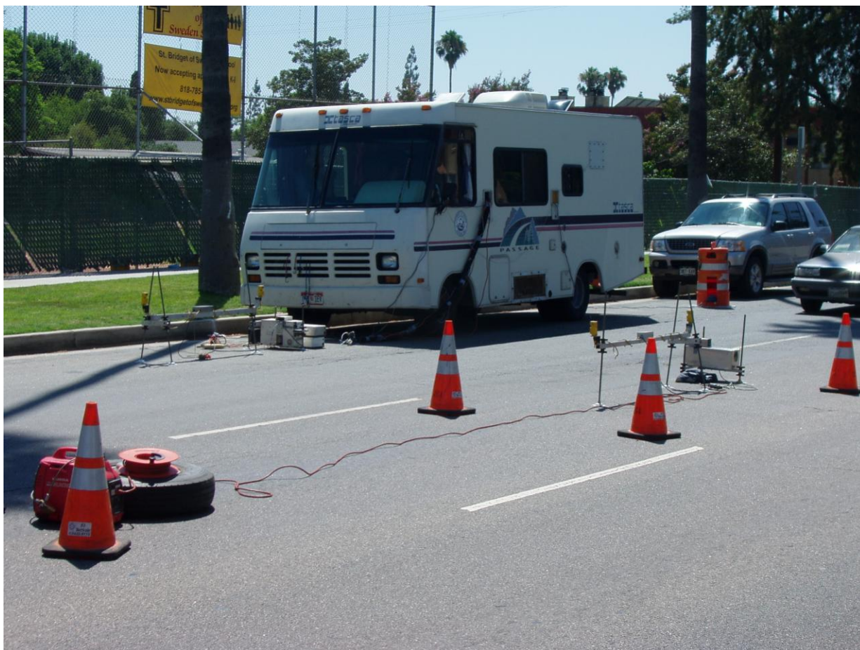
Figure 2. A street level view of the measurement setup on Sherman Way in Van Nuys CA. Across the road are the detector unit, dual spectrometers, speed bars, and the camera is in the road barrel located behind the motor home. The source, speed bars and generator are located in the closed middle lane, and the tire located next to the generator serves as an anti-theft device.
