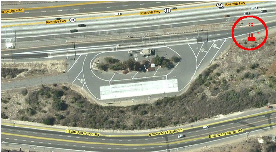
Figure 2. A satellite photo of the Peralta weigh station located on the Riverside Freeway (91). The scales are located on the inside lane next to the building in the top center and the outside lane is for unloaded trucks. The measurement location is circled at the upper right with approximate locations of the scaffolding, support vehicle and camera.
