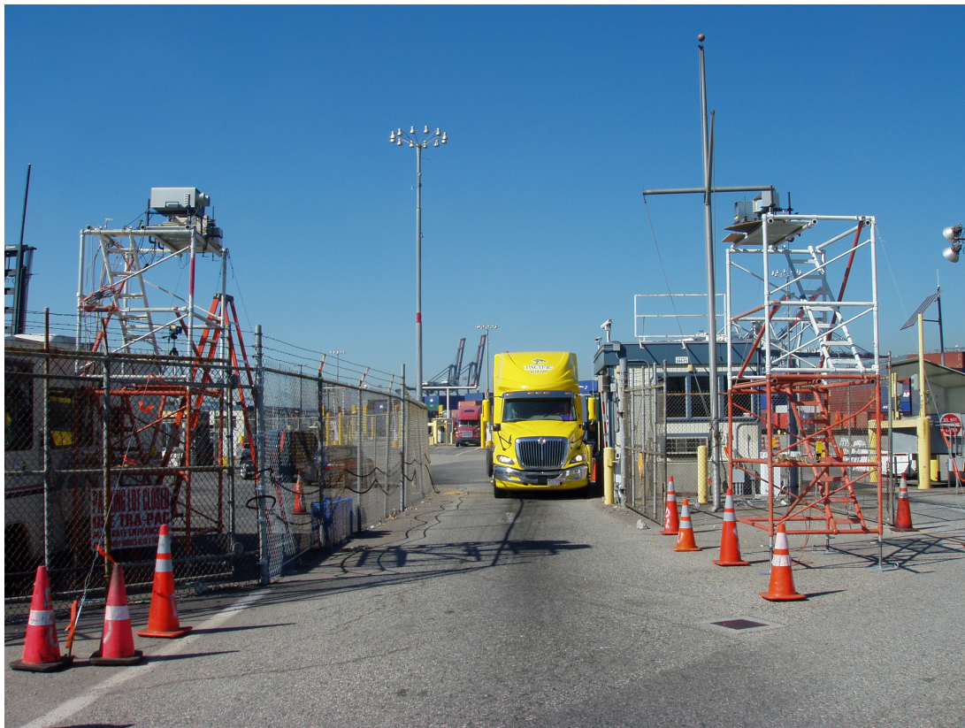
Figure 5. Photograph at the Port of Los Angeles of the setup used to detect exhaust emissions from heavy-duty diesel trucks.
