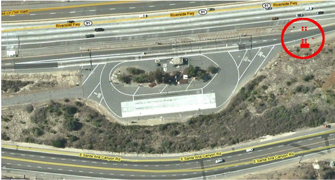
Figure 2. A satellite photo of the Peralta weigh station located on the eastbound Riverside Freeway (State Route 91). The scales are located on the inside lane next to the building in the top center and the outside lane is for unloaded trucks. The measurement location is circled at the upper right with approximate locations of the scaffolding, support vehicle and camera.
