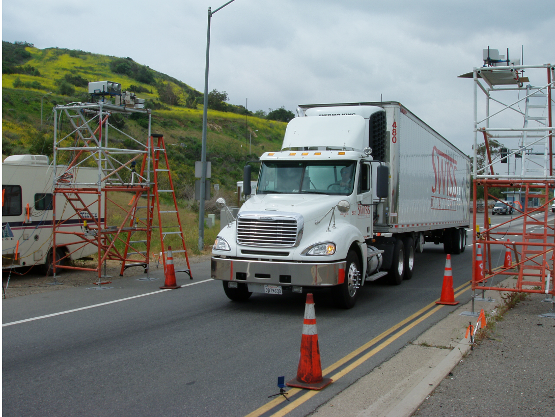
Figure 3. Photograph at the Peralta Weigh Station of the setup used to detect exhaust emissions from heavy-duty diesel trucks.
