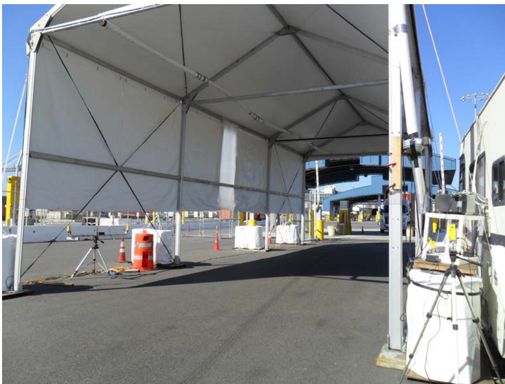
Figure 29. Photograph at the new Trapac Port of Los Angeles exit with the OHMS setup used to detect exhaust emissions from heavy-duty trucks in the foreground. The blue roofed canopies at the rear of the tent is one of the new exit check points.
