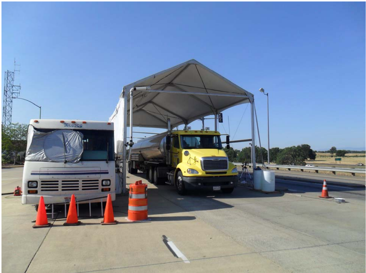
Figure 1. A photograph of the OHMS setup at the Cottonwood weigh station in northern California. The exhaust intake pipe is in the upper left part of the tent and two of the water barrels are visible next to the right front tent leg. The orange road barrel just to the right of the mobile laboratory contains the camera used to take the picture of each vehicles license plate.
