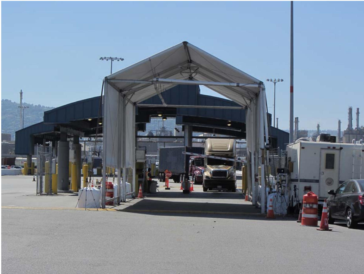
Figure 68. Photograph at the Port of Los Angeles of the OHMS setup in 2017 used to detect exhaust emissions from heavy-duty diesel trucks. The perforated exhaust sampling and integration tube is again visible on the left side of the tent and the new speed bump is located at the nearest end of the tent.
