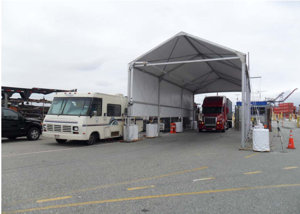
Figure 12. Photograph at the Port of Los Angeles of the OHMS setup in 2013 used to detect exhaust emissions from heavy-duty diesel trucks. The perforated exhaust sampling and integration tube is again visible on the left side of the tent.
