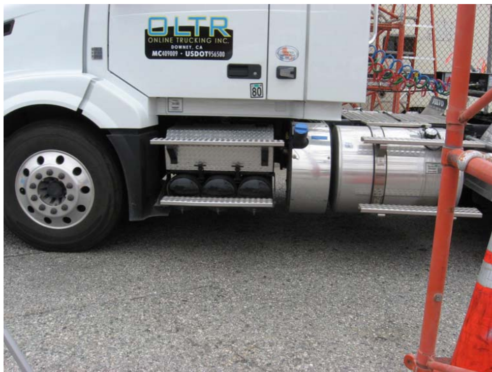
Figure 5. Driver side image of a truck leaving the port location with the urea tank clearly visible.
