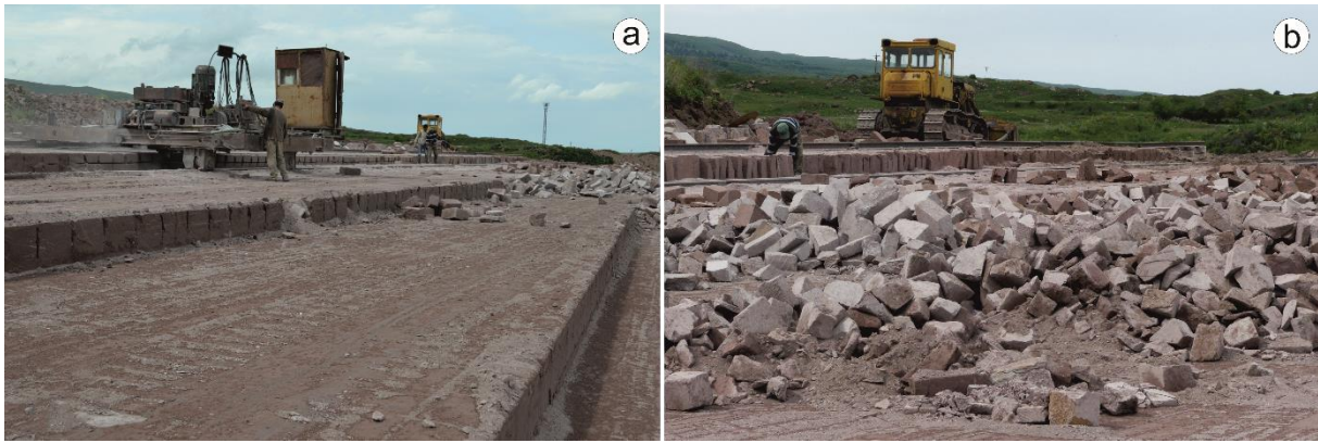
Figure 1.2: a Active tuff quarry at Mt. Aragats (Armenia). b The proportion of unusable raw blocks is very high and usually remains as large heaps at the quarry
