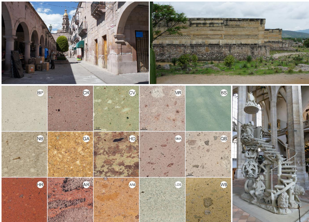
Figure 5.1: Volcanic tuffs in building heritage. Top left: the city center of San Miguel el Alto, Mexico; top right: the 2 nd century Mitla Pyramids, Mexico; bottom right: the 16 th century tulip pulpit in the Freiberg Cathedral, Germany; bottom left: macro photographs (6 x 6 cm) of the fifteen tuffs investigated in this study
