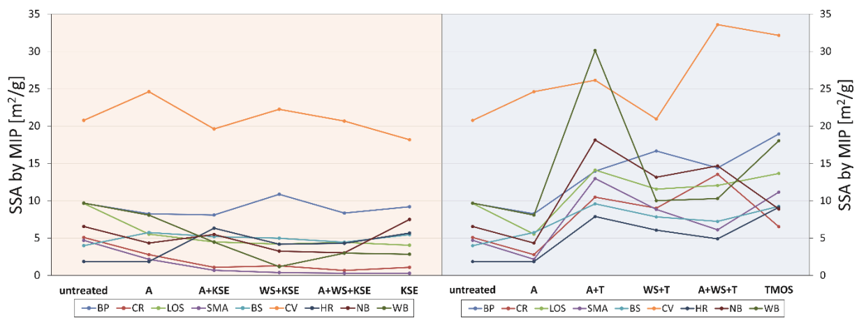
Figure 7.9: Modification of the specific surface area (SSA) due to the consolidation treatments, derived from the mercury intrusion porosimetry (MIP). Left) TEOS, right) TMOS
