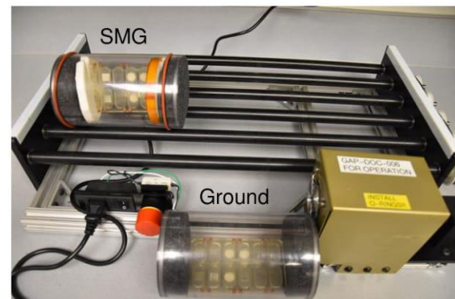
Fig. 2. BioServe's BioCells on the clinostat experiencing simulated microgravity (SMG) and respective static controls (Ground). The BioCells are placed within the Group Activation Pack (GAP). Within each well are placed the coupons: cellulose membrane and aluminium.
