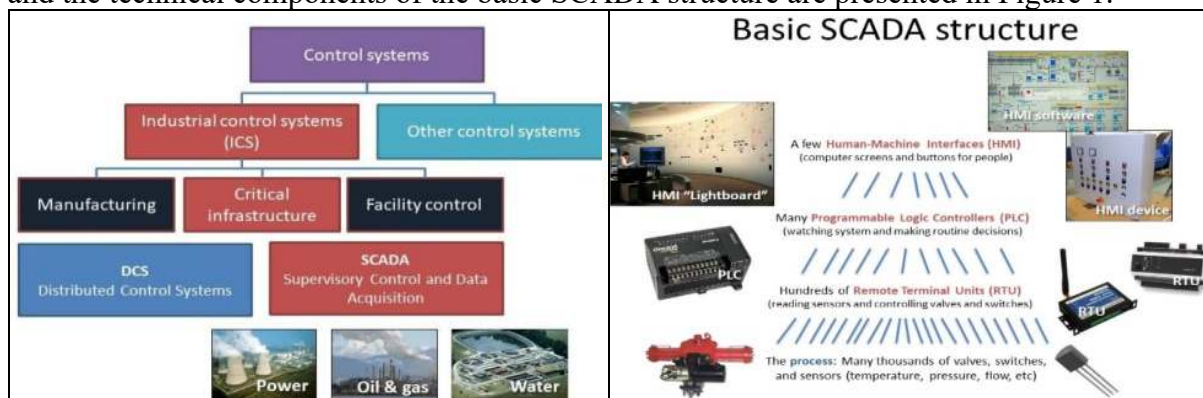
Figure 1. Use and technical components of a SCADA system.
