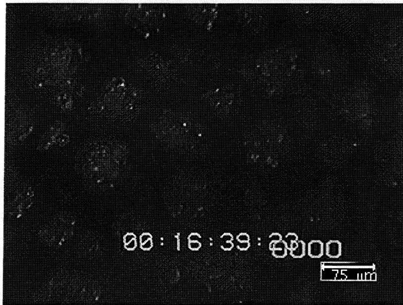
Figure 6.3 Early growth of frost on PTFE substrate, free convection
