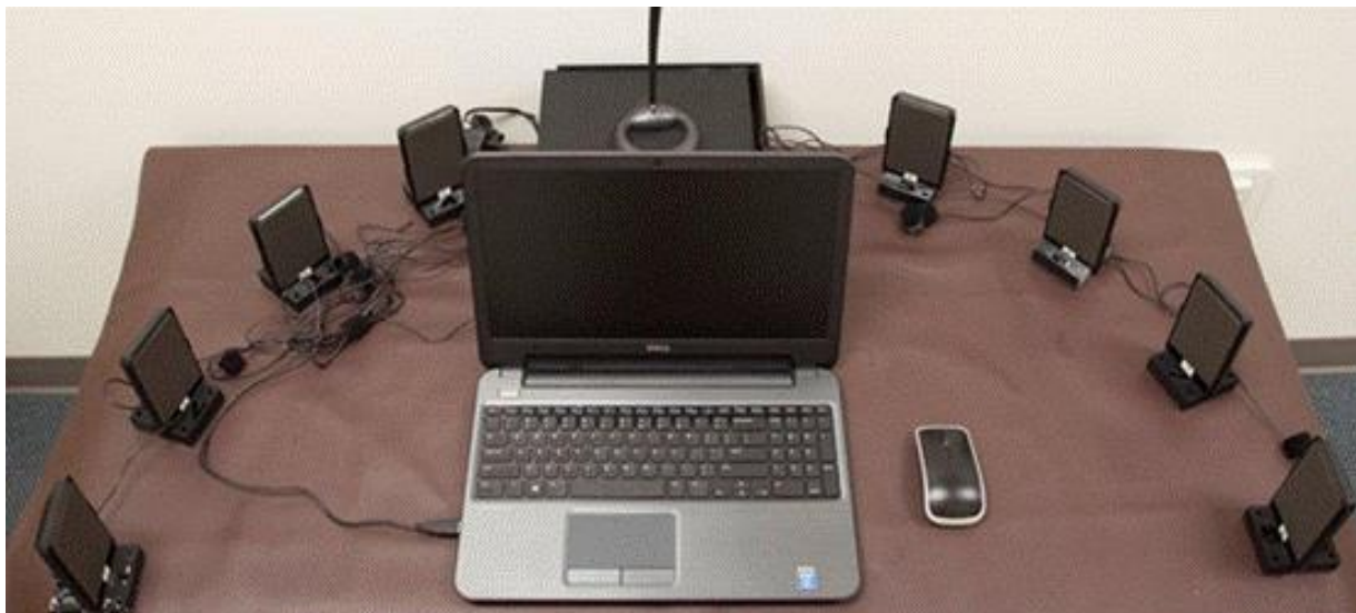
Figure 1: Photo of the computer and speaker system used by the subject to complete the Sound Localization Accuracy and Speech Understanding in Noise tasks.
