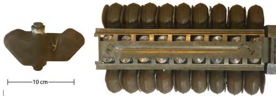
Figure 1. Diagram of individual PFM-1 anti-personnel landmine alongside KSF-1 dispersal cassette (adapted from de Smet et al. 2018). All figures courtesy of the authors.
