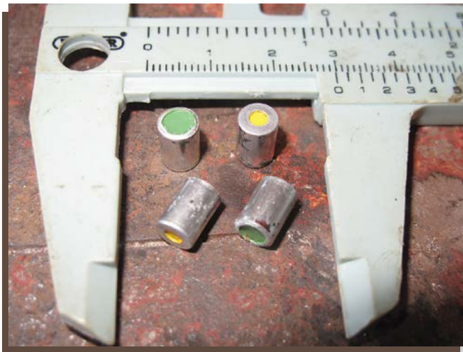
Image 10. Detonators from the SB-33 mines appeared virtually as-new, and were fully functional.
