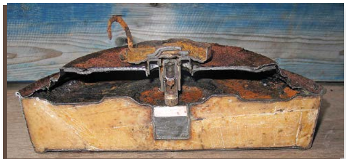
Image 7. A section through the No. 6 mine reveals that, much like the No. 4, the fuze is partially seized but the explosive train remains functional.
