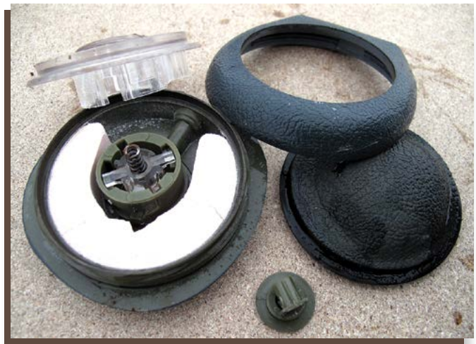
Image 8. A disassembled Italian SB-33 mine, showing most components in good condition.
