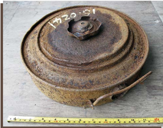
Image 6. The heavily rusted casing of the Israeli No. 6 AT mine.
