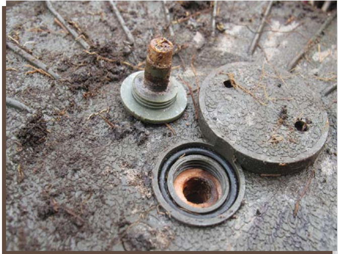
Image 13. The stab-receptors of the SB-81 detonators were no longer functional.
