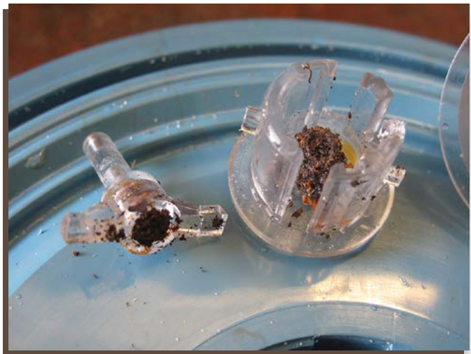
Image 12. The SB-81 striker springs had rusted away.
