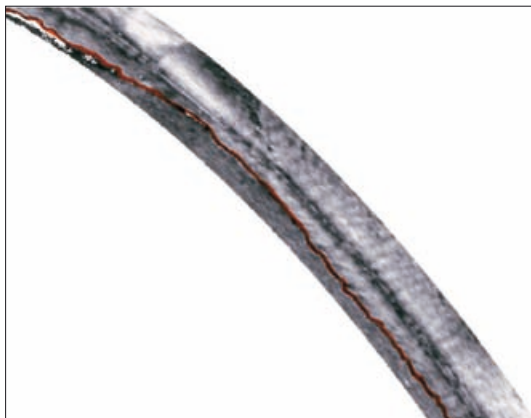
Fig. 2: Section of AUV side-scan showing bedforms and river bank triple points (highlighted in red)
