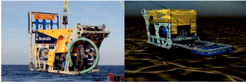
Fig. 4: Heavy duty work class ROVs
