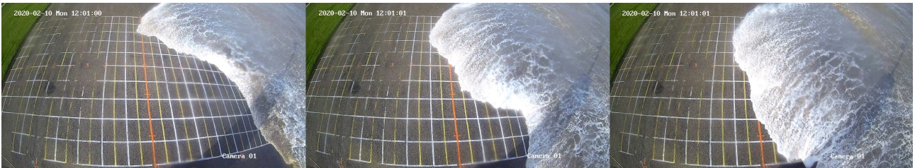
Figure 5: Three snapshots taken from the video recordings, showing a very oblique wave running up the slope in a sort of local plunging motion. Note the painted grid as used for the video analysis.
