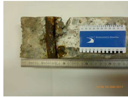
Figure 4: Drilled core no. 4, 1st and 2nd layer of rebars (left); drilled core no. 4, split, 1st and 2nd layer of rebars (right)
