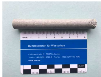
Figure 6: Drilled core no. 1, after sampling, 1st layer of rebars, width of crack at surface approx. 0.25 mm, concrete cover approx. 60 mm (left); drilled core no. 1, rebar in first layer after application of the pickling solution, minor reduction in the cross-section at the right-hand edge (right)
