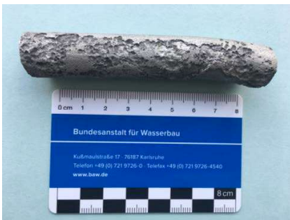
Figure 5: Drilled core no 4, rebar in 1st layer after application of the pickling solution, extensive erosion (left); rebar in 2nd layer after application of the pickling solution, no reduction in the cross-section (right)
