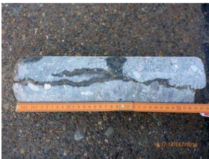
Figure 6: Drilled core no. 1, after sampling, 1st layer of rebars, width of crack at surface approx. 0.25 mm, concrete cover approx. 60 mm (left); drilled core no. 1, rebar in first layer after application of the pickling solution, minor reduction in the cross-section at the right-hand edge (right)
