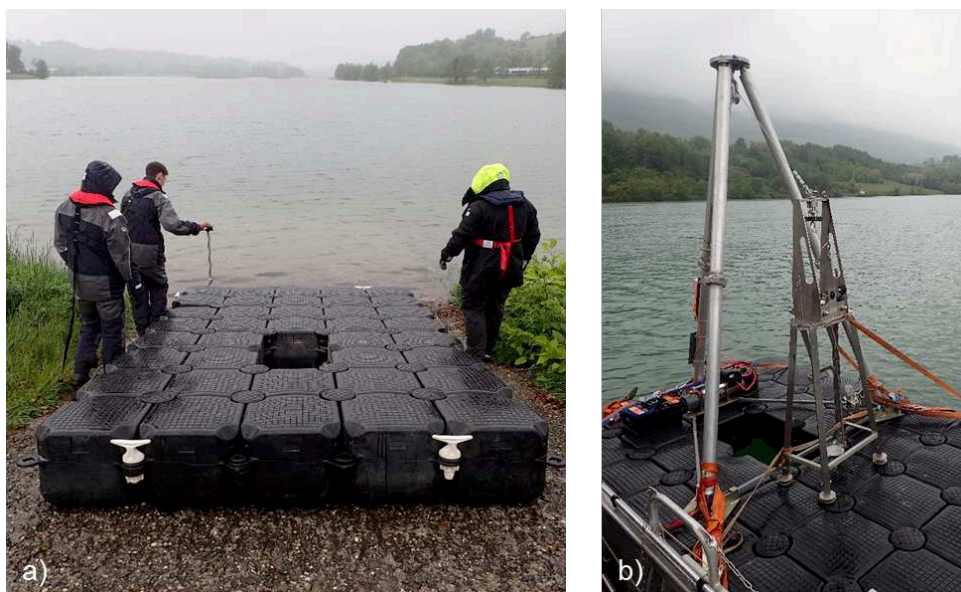
Figure 3.2. Platform used to operate the Frahm Sediment Sampler (a) after assembly on land, (b) completely equipped with tripod, electric winch, and Frahm Sediment Sampler (on rack) on the water (Beckers et al., 2019).
