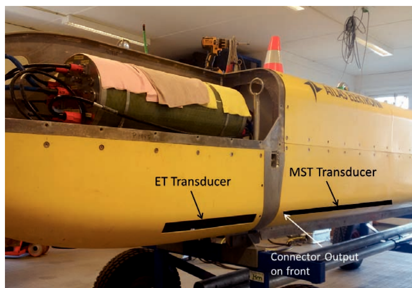
Fig. 1: Mounting of the sonars on the AUV
