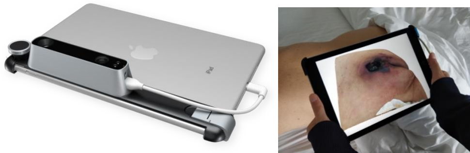
Figure 27: Left: The Structure Sensor mounted on an iPad. Right: Scanning of a pressure injury using the Structure Sensor
