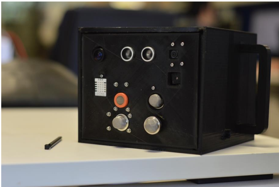
Figure 47: The device for pressure injury data acquisition
