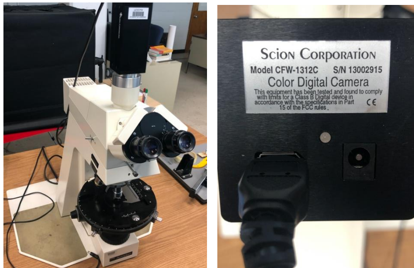
Instrumentation used for whole-thin section imaging to produce base map mosaics: Zeiss Axioplan optical microscope fitted with a Scion Corporation CFW-1312C Color Digital Camera, housed in the Department of Geography and Geosciences at the University of Louisville.
