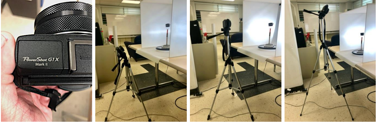
Instrumentation used in billet imaging for SFM reconstruction: Canon Powershot G1 X Mark II digital camera, adjustable camera tripod, desktop light diffusing tent, and custom-made sample mount.
