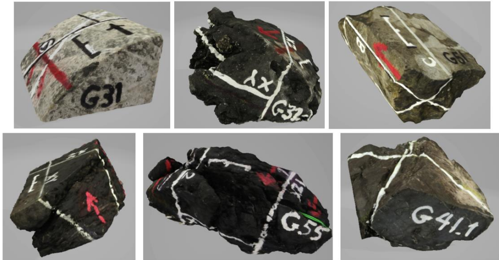
Figure 15. Illustration containing 6 finalized solid surface models, indicating various combinations of the discussed billet reference markings and SFM's flexibility given a wide range of billet composition and geometries.
