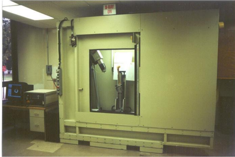
Figure 10: ACTIS high resolution computed tomography (HRCT) laboratory scanner used in the current study
