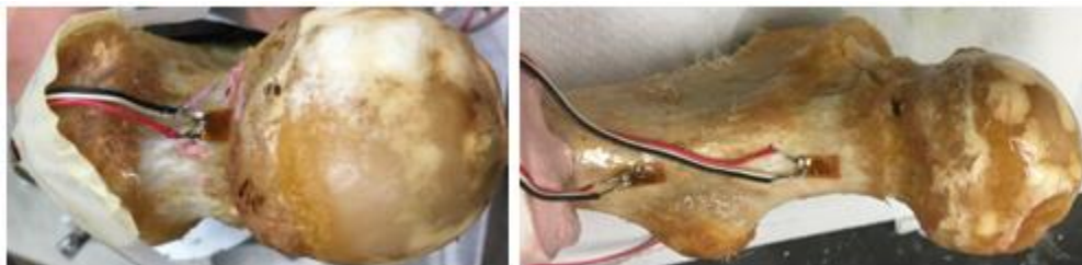
Figure 41: A strain gauge was placed on the superior neck of the cadaveric femur on the left. The other two strain gauges were placed on the inferior neck and the medial shaft
