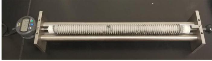
**Fig. 5.4.** Dilatometer with corrugated mould for linear autogenous strain measurement
