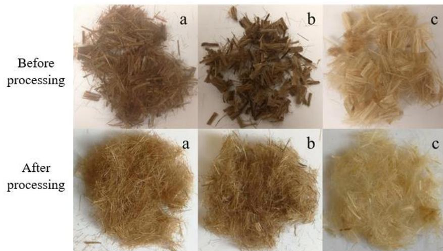
**Fig. 5.2.** Kenaf fibers before and after processing: (a) RKF; (b) AKF; (c) AHPKF
