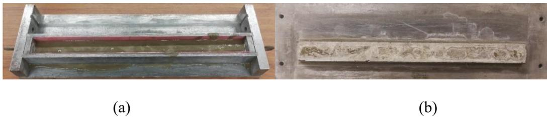
**Fig. 5.6.** Sample (a) casting and (b) demolding
