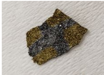
Figure 50. \text{GaSb}_x\text{P}_{(1-x)} with 4 thermally evaporated Sn/Au contacts before annealing.
