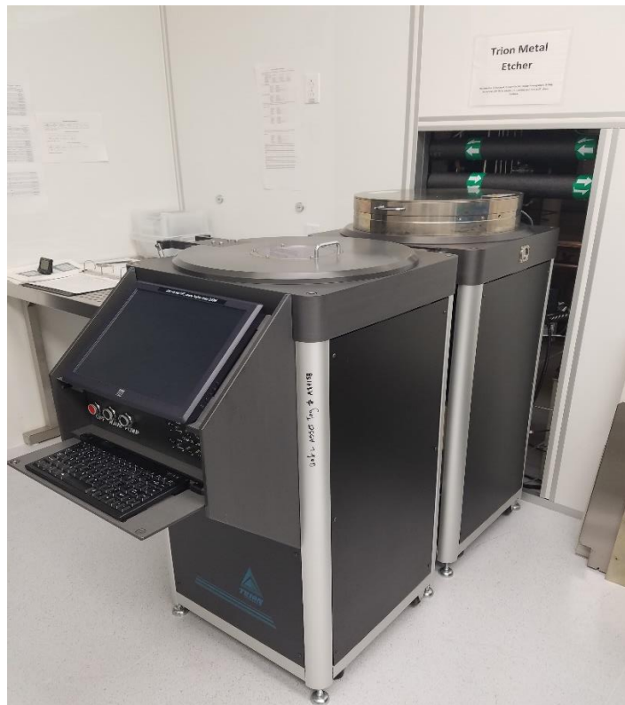
Figure 57. ICP/RIE Trion Metal Etcher located in the etching bay at the UofL Micro/Nano Technology Center.
