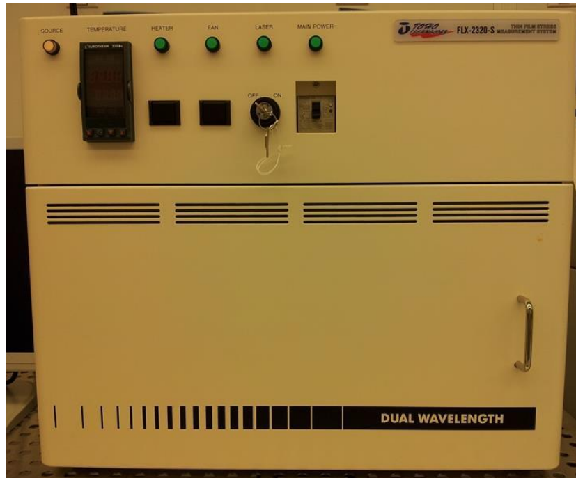
Figure 56. Toho FLX-2320-S thin film measurement machine located in the deposition bay at the UofL Micro/Nano Technology Center.
