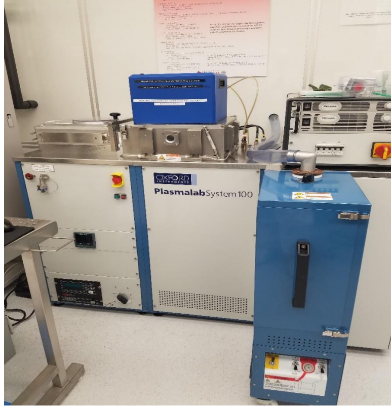
Figure 55. Oxford PECVD PS100 machine located in the deposition bay at the UofL Micro/Nano Technology Center.
