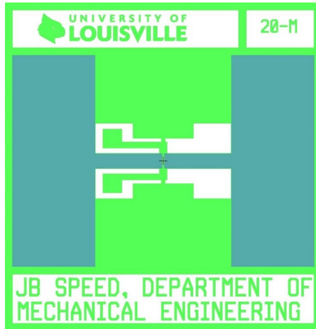
Figure 47. The photomask layout corresponding to the molybdenum as the bottom electrode layer of the device.
