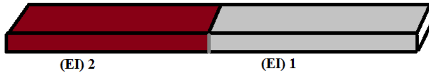
Figure 7. A schematic view of a single beam with different material properties.
