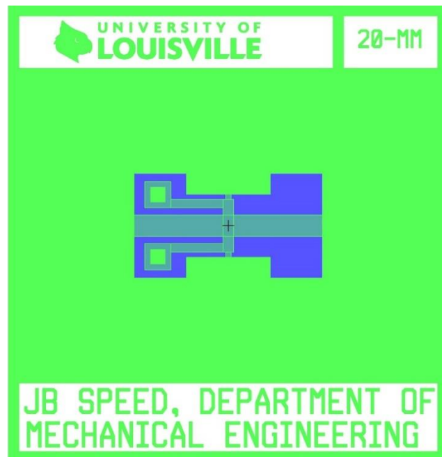
Figure 50. The photomask layout corresponding to the bulk etching of the top fabricated device in the DRIE process.
