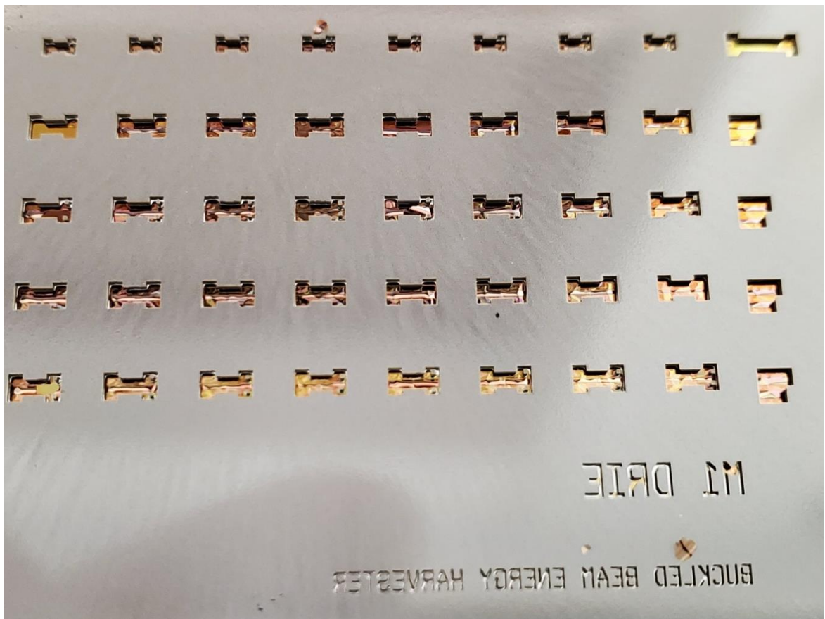
Figure 63. Backside view of the fabricated wafer after the DRIE process.
