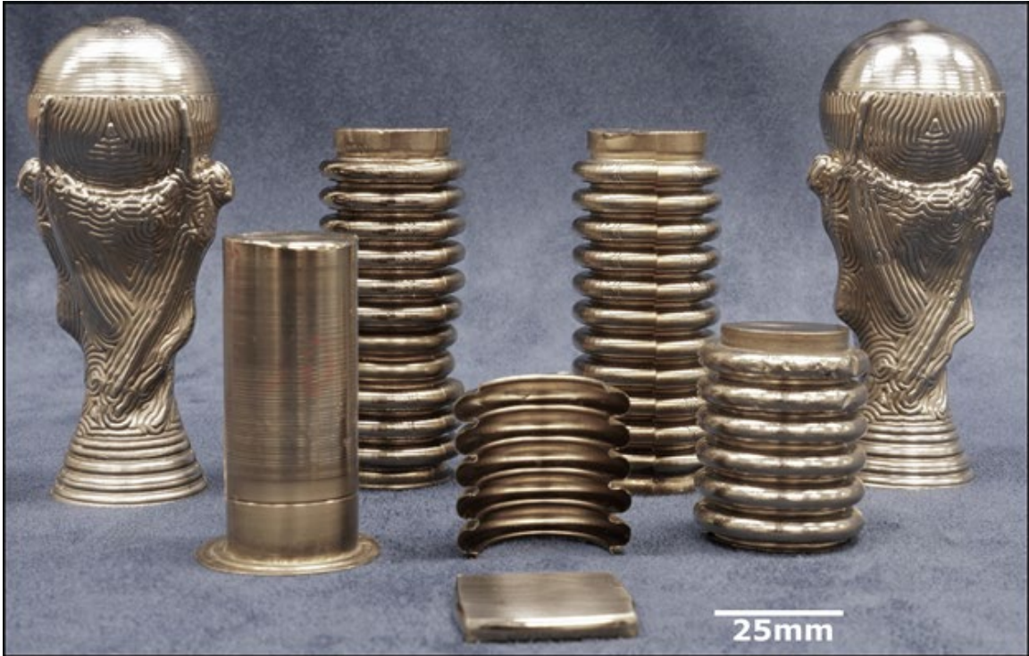
Figure 34. Parts obtained through the stretch blow molding process. By starting with a flat sheet-like feedstock with a few mm in thickness as the one shown at the center of the image parts with aspect ratios of 4 and strains over 2000% were obtained.
