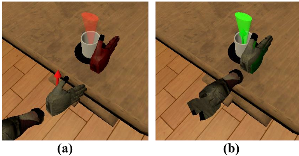
Fig 4.5 – Example of a reach to a cup task. (a) Semi-transparent hand indicates the desired goal position of the user-controller hand, which dims as the hand approaches it. A red arrow is included next to the hand to assist with visualizing the current hand orientation. (b) Task completion occurs when the hand is within the Euclidean tolerance and the corresponding orientation arrow is within the tolerance cone.
