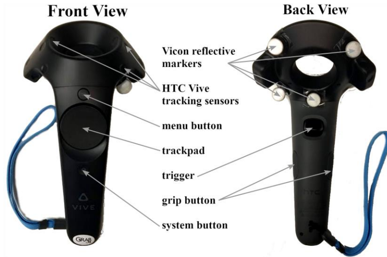
Fig 4.3 – Standard HTC Vive Controller. Vicon reflective markers were placed in a known arrangement around the controller’s head and were used to calibrate the virtual space between Vicon and HTC.
