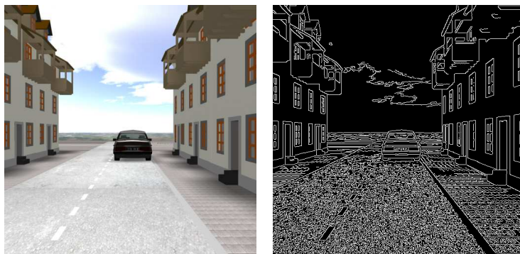
Figure 4: (left) Left image of the stereo pair #293 of the virtual stereo sequence and (right) its corresponding edge image.
