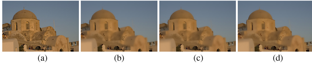
Fig. 2 Example bilateral filtering results. (a)–(d) Parameters were \gamma = 10 , \phi = 51 , W = 61 . (a) Input image, (b) BF (61.98 s), (c) BF implementation 16 (2.96 s), and (d) proposed CCBF (0.93 s, with M = 31 , #conv = 62). Iteration numbers were chosen to yield PSNR \geq 41.14 dB relative to the BF output. Image 11 ( 876 \times 584 \times 3 ) with 8-bits per pixel.
