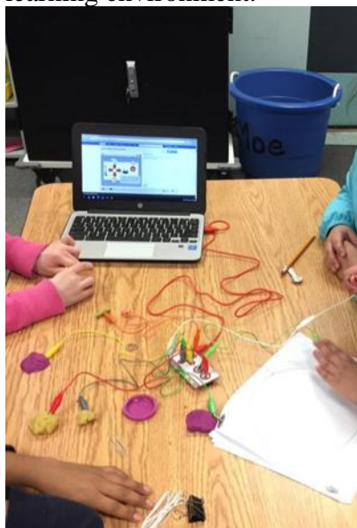
Figure 2. Using a Makey Makey to test playdough and graphite for conductivity.
