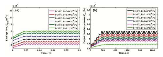
Fig. 3 — Effect of temperature on (a) Leakage flow, (b) Output piston chamber pressure
