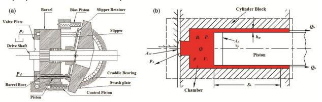
Fig. 1 — Schematic system diagram (a) Axial piston pump considered under study, (b) Control volume for the development of pressure in the piston chamber
