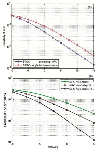
Fig. 2 — (a) Performance analysis of MRC with single relay, and (b) performance analysis of MRC by changing the number of relays.
