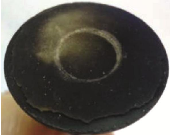
Fig. 7 — valves after 60 hours of operation
