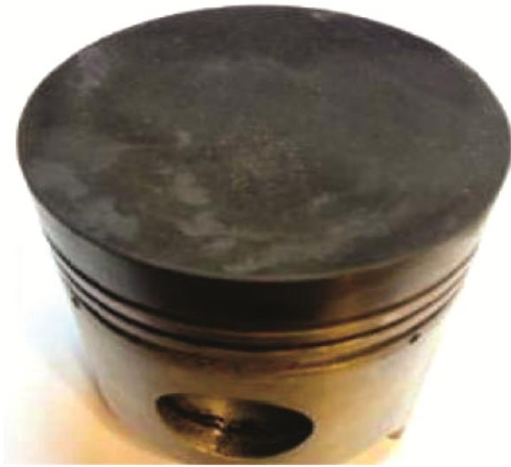
Fig. 8 — State of the coating after 60 hours
