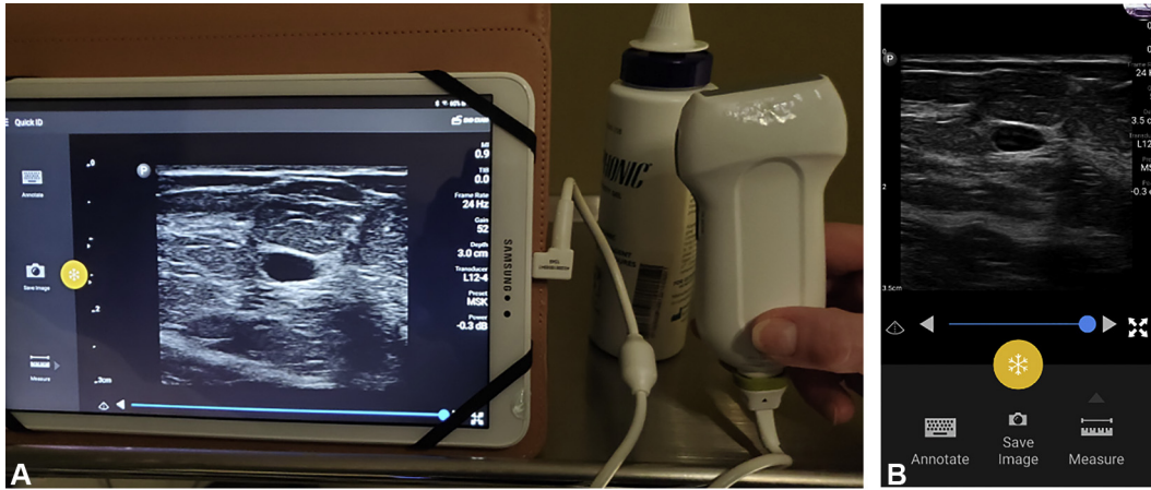
Figure 1. (A) Phillips Lumify Tele-Ultrasound Linear Ultrasound Transducer Probe; (B) Smartphone Enabled Ultrasound demonstrating image quality with both smart pad and smart phone.
