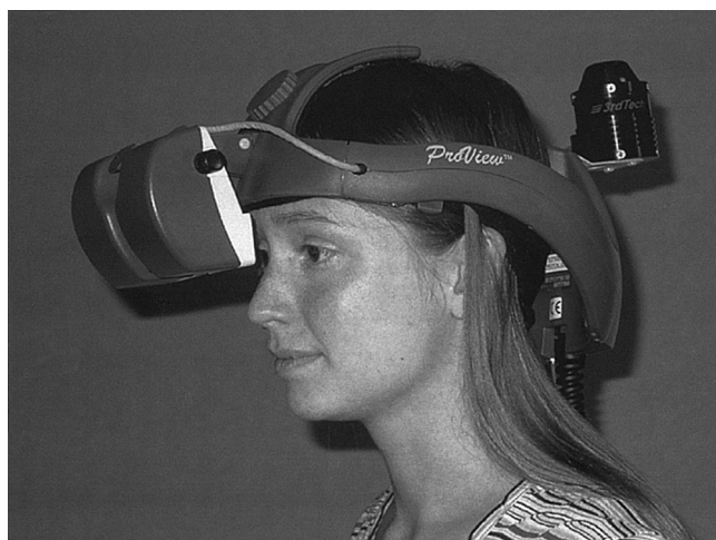
Figure 4. A user wearing the HMD component of our prototype hybrid display with an attached HiBall tracker sensor (Welch et al., 2001).
