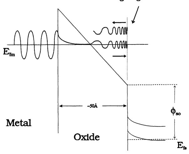
Electrons can coherently reflect off of Si/SiO<sub>2</sub> Interface.
